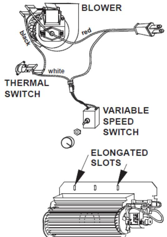
Tilt the blower onto its side. Slide it past the controls and into the clip **(C)**. Secure to the threaded stud using the lock washer and wing nut provided. Ensure that the blower does not touch the fireplace base or the firebox.
