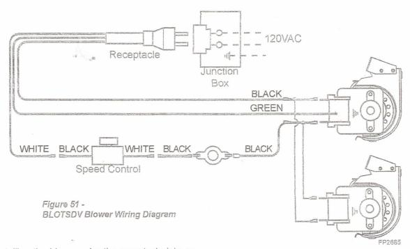
Before installing the blower, wire the receptacle into an electrical circuit. This should be done before framing the fireplace. Wire with minimum 60° C wire in accordance with prevailing codes.
